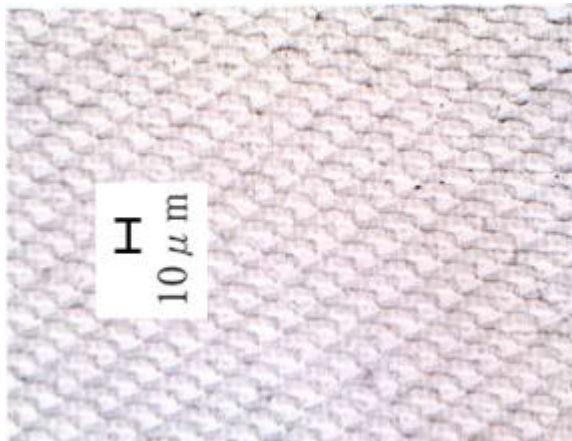
a) s=1500\text{rpm} , f=7.5\text{mm/min} ( =5\text{ }\mu\text{m/rev} )
