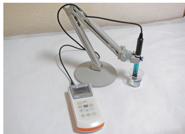
図6 塩化物イオン濃度計測に用いた機材 Fig. 6 A device used to measure chloride ion concentration
