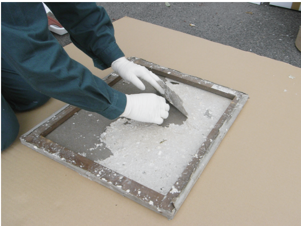
図3 裏面に付着した流出バルブの除去 Fig. 3 Removing runoff pulp attached to the back side
