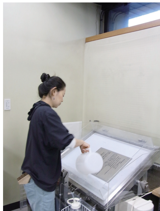
図6 漉きばめ機を使った作業 Fig. 6 Repair process using a leaf casting machine
